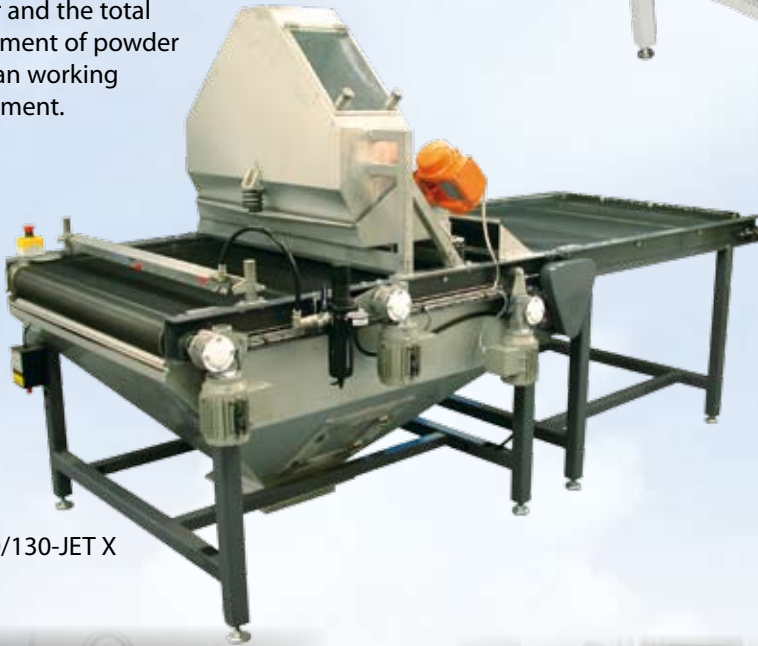
Spreading a uniform layer of powder
