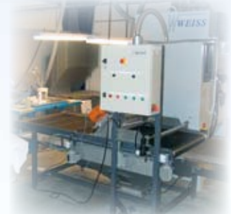
Spreading a uniform layer of powder
